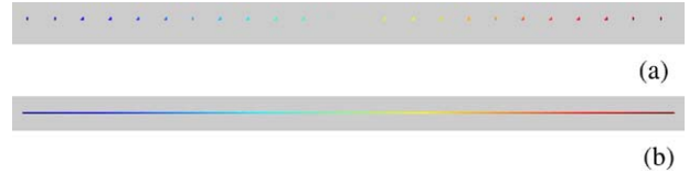
Fig. 4. A univariate heterogeneous lofting example. (a) Profile points. (b) Lofted heterogeneous curve.
