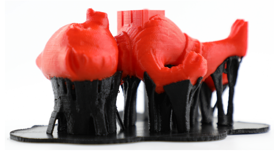
(b) Side view of 3D printed part with optimized supports
