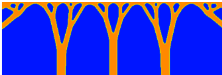
Figure 7: Optimized supports in a 1 \times 1 rectangular domain with 0-displacement boundary conditions on different parts of the boundary. In all cases, the optimized designs are self-supporting
