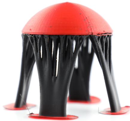
Figure 17: 3D printed optimized supports for a tall dome (printed in an Ultimaker 3)
