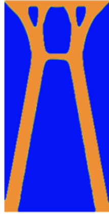
(a) Supports without overhang constraint
