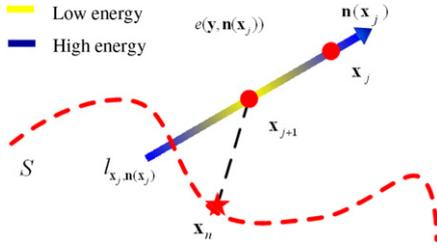
Fig. 2. Illustration of the MLS projection process.
