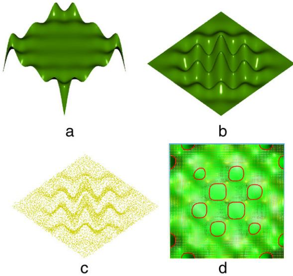
**Fig. 16.** Intersection of NURBS surface A and Point-set surface C. (a) NURBS surface A. (b) Nominal NURBS surface B. (c) Point-set surface C generated from surface B by sampling  $100 \times 100$  points and by adding random noise with a standard deviation of 0.1. (d) Intersection result.
