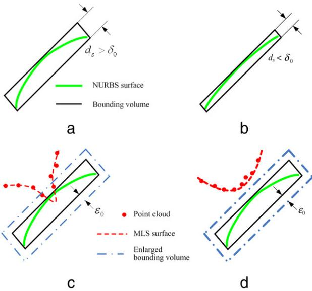
**Fig. 11.** Two criteria for leaf node identification in quad-tree construction. (a) The patch needs to be further subdivided due to the larger planar distance of the bounding volume according to the 1st condition. (b) The patch is identified as a leaf patch due to the smaller planar distance of the bounding volume according to the 1st condition. (c) The patch needs to be further subdivided according to the 2nd condition. (d) A patch is identified as a leaf patch according to the 2nd condition.
