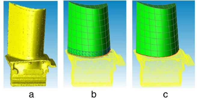
**Fig. 15.** Example 3: Boolean operation of a NURBS “airfoil” and a point-set “platform”. (a) Iso-view of a whole scanned turbine blade. (b) Iso-view of the platform of the scanned turbine blade and a newly designed airfoil. (c) Iso-view of the Boolean result.
