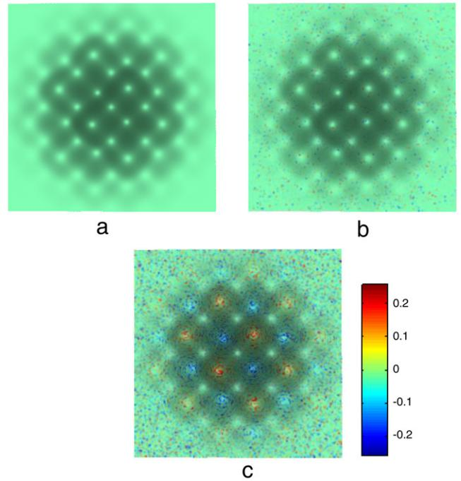
**Fig. 17.** Error distributions between nominal NURBS surface B and MLS surfaces with different Gaussian factor  $h$ . (a)  $h = 0.03$ . (b)  $h = 0.3$ . (c)  $h = 3.0$ .
