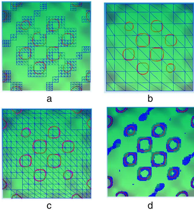
**Fig. 18.** Intersection results with different  $\delta_0$  and  $\varepsilon_0$ . (a)  $\delta_0 = 0.3$ ,  $\varepsilon_0 = 0.0$  (broken inner intersection curves). (b)  $\delta_0 = 1.2$ ,  $\varepsilon_0 = 0.3$  (missing boundary intersection curves). (c)  $\delta_0 = 0.6$ ,  $\varepsilon_0 = 0.3$  (correct topology and poor accuracy). (d)  $\delta_0 = 0.03$ ,  $\varepsilon_0 = 0.3$  (correct topology and good accuracy).
