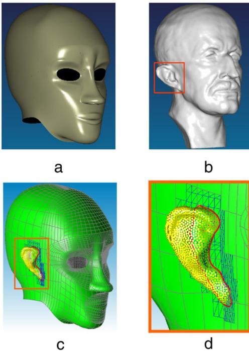
**Fig. 14.** Example 2: Intersection of a NURBS “head” and the point-set “Max Planck bust’s ear”. (a) Original NURBS surfaces of a head. (b) Original point-set surface of Max Planck bust. (c) Intersection result. (d) Zoom-in to the intersection region.
