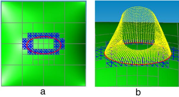
**Fig. 10.** Adaptive subdivision of a NURBS surface ensuring accurate and efficient NURBS/MLS surface intersection: Patches closer to the intersection curves undergo more times of subdivision. Planar triangles are only generated from the leaf patches that can potentially intersect with the MLS surface. (a) Top-view. (b) Iso-view. (For interpretation of the references to colour in this figure legend, the reader is referred to the web version of this article.)
