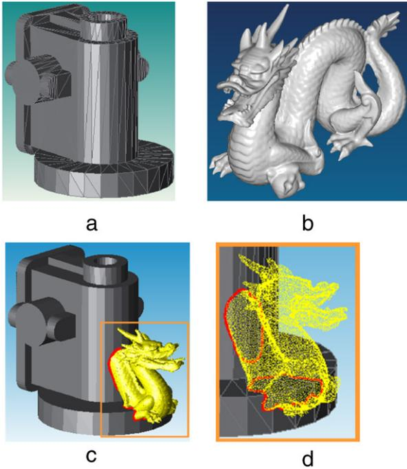
**Fig. 13.** Example 1: Intersection between polygonal and point-set surfaces. (a) Triangular mesh of a reducer. (b) Point-set surface of a dragon. (c) Left-front-view of the intersection result. (d) Zoom-in of the result in (c).
