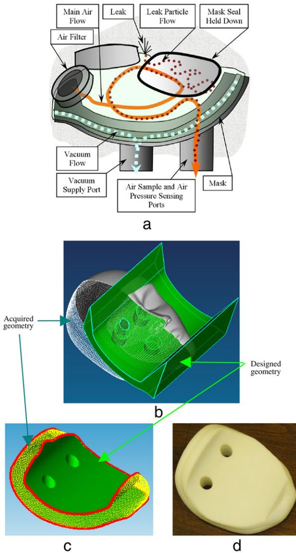
**Fig. 1.** Designing and manufacturing of a customer-specific headform: (a) Physical mask, (b) Acquired head model and the designed mask template. (c) Direct Boolean intersection result. (d) Rapid prototyped part from the intersection resulting model.
