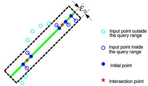
Fig. 3. Strategy for generating different initial points for locating multiple line/MLS surface intersection points: points that are  $\varepsilon_0$  distance away from the line are projected onto the line and the projected points are then used as the starting points to find the intersection points between the line and the MLS surface. (For interpretation of the references to colour in this figure legend, the reader is referred to the web version of this article.)
