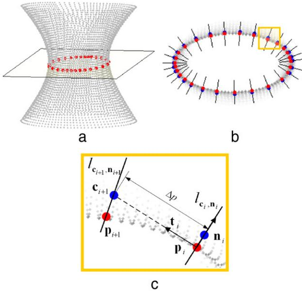
**Fig. 5.** Illustration of adaptive marching in plane/MLS surface intersection. (a) Iso-view of a point data with resulting 2D contour on a slicing plane. (b) Top-view of the slice at  $z = 0.1$ . (c) Zoom-in.
