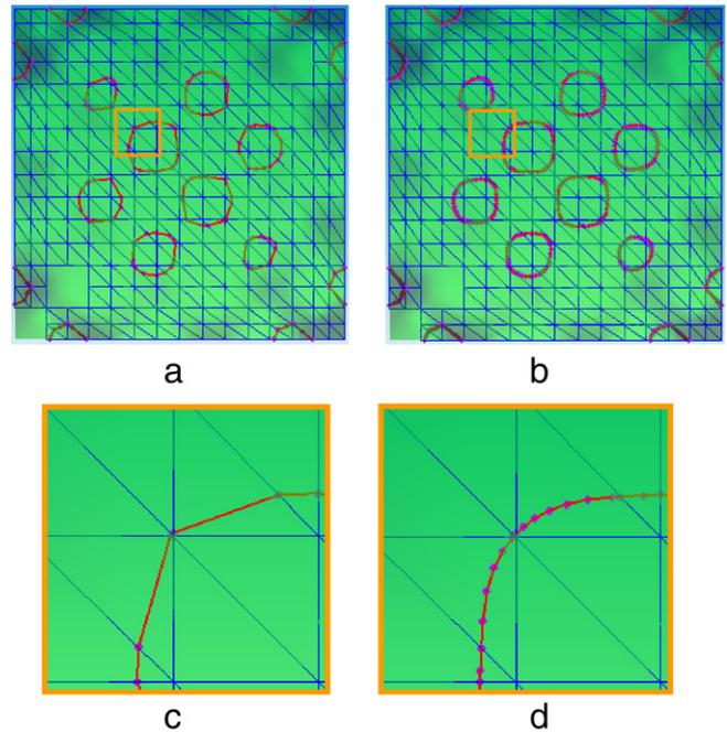
**Fig. 19.** Intersection results with different  $\delta_s$  ( $\delta_0 = 0.6$ ,  $\varepsilon_0 = 0.3$ ). (a)  $\delta_s = 0.03$ . (b)  $\delta_s = 0.003$ . (c) Zoom-in of (a). (d) Zoom-in of (b).
