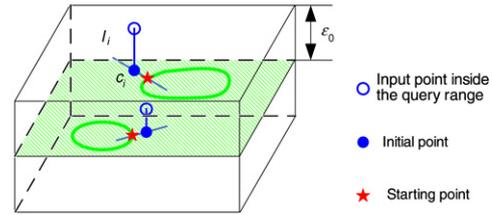
Fig. 4. Strategy for locating the starting points for the marching process in plane/MLS surface intersection: points that are  $\varepsilon_0$  distance away from the plane are projected onto the plane and the projected points are then used as the initial points to find the intersection points between the line and the MLS surface. These intersection points become the candidate starting points for the marching process.
